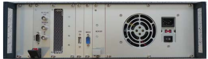
The rear of the instrument contains all necessary connectors for inputs and communication interfaces.
