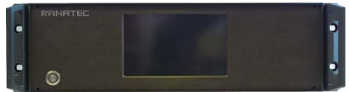
Ranatec RI 900 is a modular Radar Performance Monitor for online measurements.
